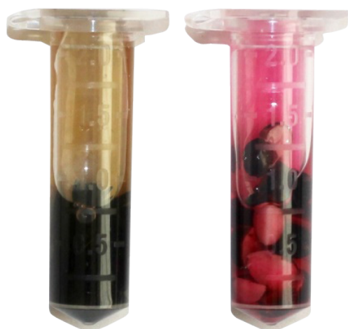
Fig. 2. Qualitative testing vetch seed pigments by soaking crashed seeds in basic (left tube) and acidic (right tube) solutions
